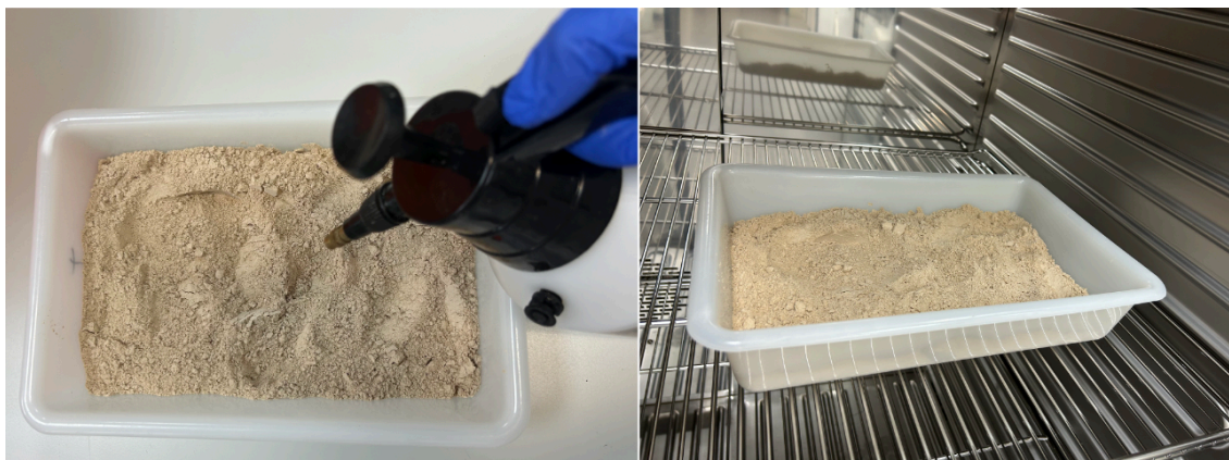
Figure 1. Treatment of fibrous ingredients with multi-enzymatic complexes by the solid-state hydrolysis (SSH) procedure. Application of the enzymatic complex (left) and hydrolysis incubation under optimal conditions (right).
