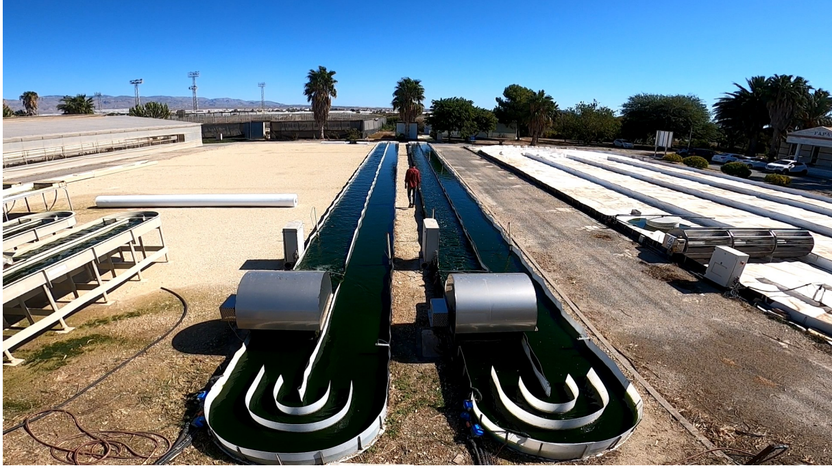
Figure 2.14. Microalgae raceway reactor located at the IFAPA center, close to the University of Almería.
