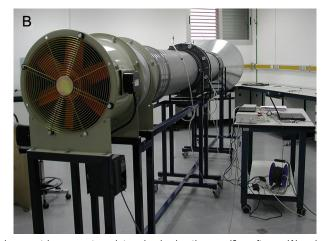
Figure 2 – Digital microscope image of the mesh used as a windbreak and geometric parameters determined using the specific software (A) and wind tunnel used for the aerodynamic characterization of the mesh (B).
