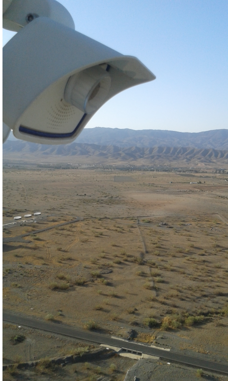
Figure 3: One of the six shadow cameras overlooking the PSA from top of a tower (CIEMAT CESA-I), 87 m above the ground.
