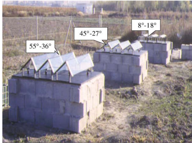
Fig. 1. East–west oriented 1:15 greenhouse models at the experimental site (latitude 37^{\circ} 10'N ), south of Spain, with the south-facing and north-facing slopes shown for each model
