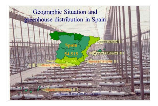
In the Mediterranean area and Canary Islands, hundreds of Has of land are covered with polyetilene film, supported by wooden or iron posts to form a single greenhouse structure called "parral" or "arbour" greenhouse
