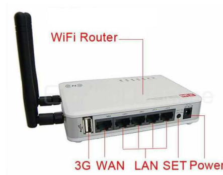
Figura 3.23: Router SL-R7205 11N 300M (OpenWRT)
