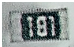
Figure 54 – Photograph of the resistance used for the repeatability and accuracy tests
