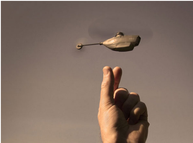
Figure 7 – Black Hornet Nano: is a micro unmanned aerial vehicle (UAV) used by British and Norwegian armies for recognition and surveillance
