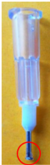
Figure 35 – Unconventional vacuum gripper: its extremity consists in a nozzle with multi-lumina. This end-effector was tested as an alternative to the one used.
