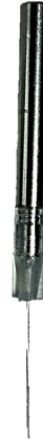
Figure 44 – Rapidograph inner needle. The mass has the same dimensions for all, while the thinner part varies.
