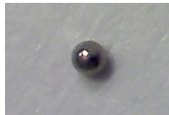
Figure 55 – Photograph of the tin sphere ( \Phi=600 \mu\text{m} ). Taken with an USB microscope.
