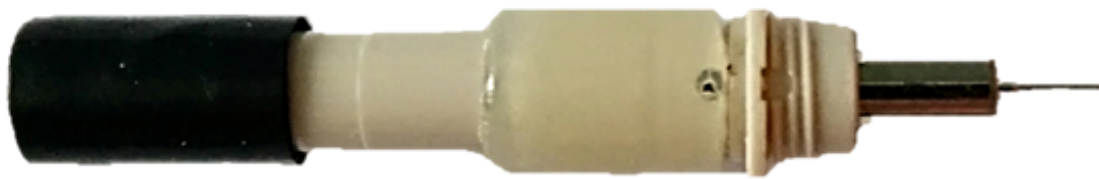
Figure 50 – Rapidograph in operative conditions: the rapidograph as shown is ready to be used on the robot as end-effector. We invite the reader to notice the little hole dug in the rubber tube in correspondence of the lateral hole of the nib. Such a hole allows enough amount of air to pass and to lift the needle, but not too much (jeopardizing the gripping force). The rubber adhesive tape permits to connect the pen to its adaptor.
