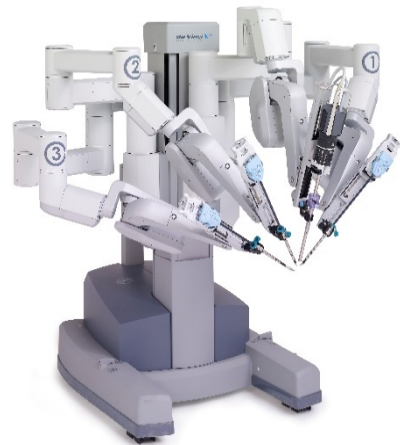
Figure 8 – Da Vinci Surgical System: surgical robot for minimally invasive operations
