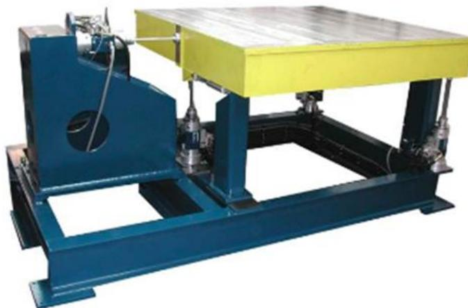
Fig. 2 11 Mesa de vibraciones Bi-axial vibration Systems de Servotest [22].
