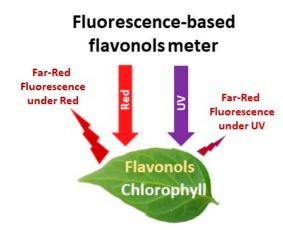
**Figure 5.** Schematic representation of the functioning of fluorescence-based flavonols meters by using the chlorophyll fluorescence screening method.
