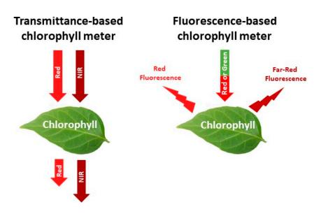
**Figure 1.** Functioning of two different types of chlorophyll meters used to estimate leaf chlorophyll content.
