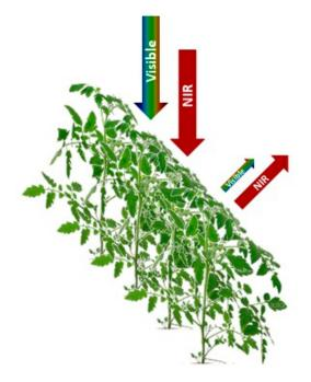
**Figure 3.** Schematic representation of the functioning of active canopy reflectance sensors. Differential reflectance of visible and near-infra red radiation (NIR) is used to calculate vegetation indices.
