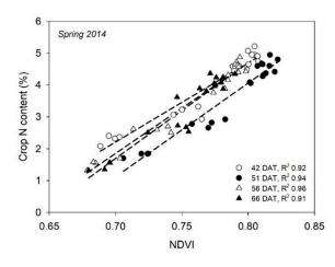
**Figure 4.** Linear relationships of the Normalized Difference Vegetation Index (NDVI), measured in the upper part of the crop canopy with a Crop Circle ACS 470 sensor, to standing crop N content from a greenhouse-grown cucumber crop in Spring 2014 carried out in southeast Spain. DAT is days after transplanting and  $R^2$  is the coefficient of the determination of linear regression.
