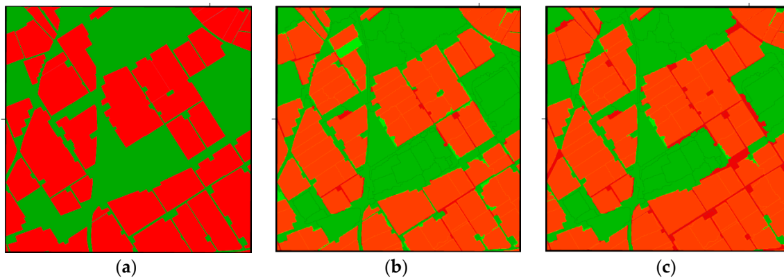
Figure 8. Pixel-based accuracy assessment for the developed DT models over the same detailed area used in Figure 5 (1000 m \times 1000 m): (a) Manually digitized ground truth; (b) Classification results using the DT model for S2A; and (c) Classification results using the DT model for L8. The GH class is represented in red, and the Non-GH class is represented in green. Light green and brown colors in both classification maps highlight the misclassification errors.
