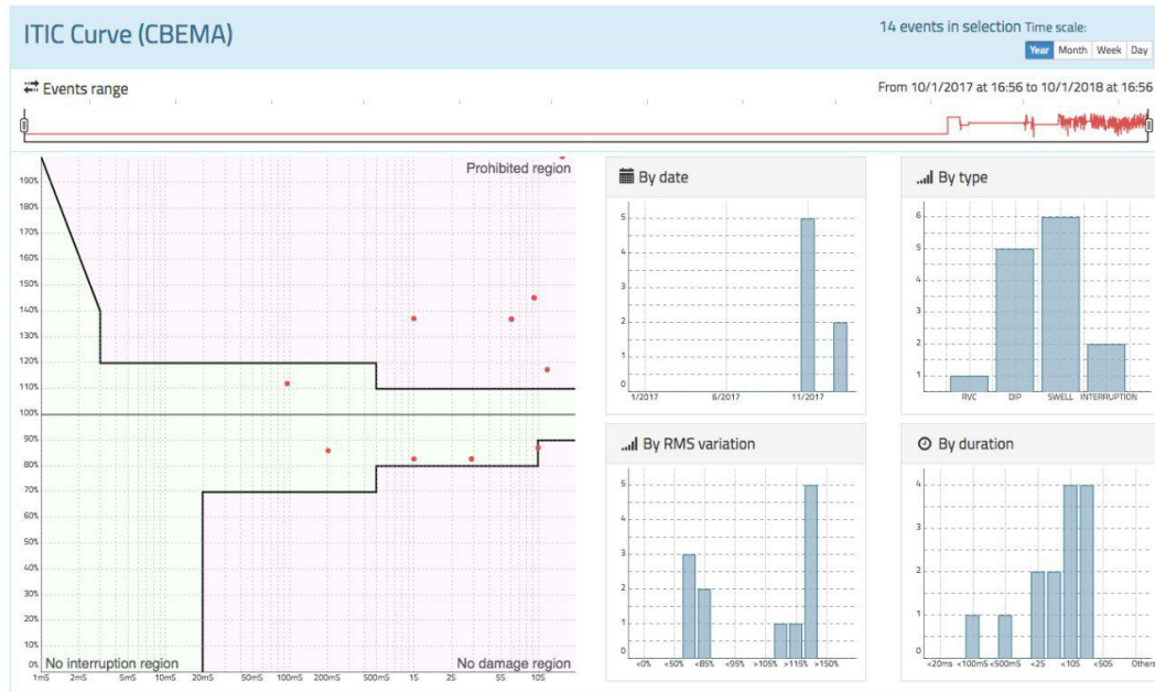
Figure 6. The ITIC (CBEMA) curve in the oZm graphical interface.
