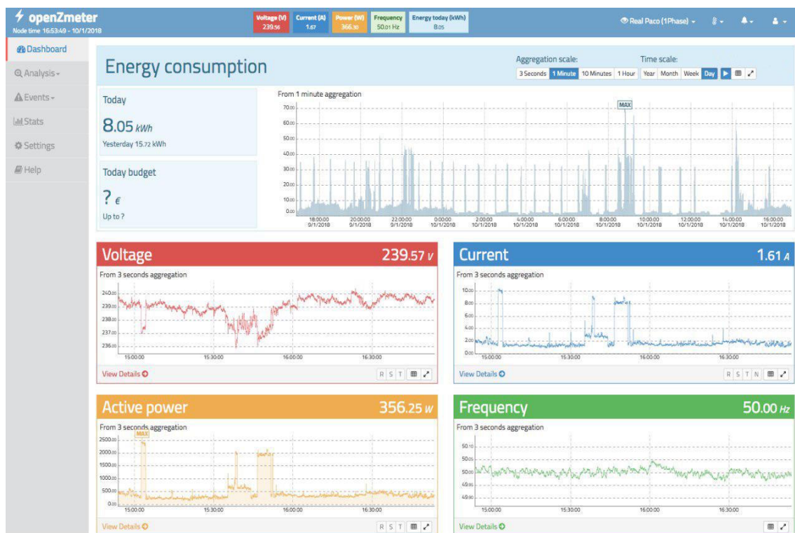
Figure 3. Dashboard of oZm. From top to bottom and left to right, active energy, RMS voltage, RMS current, active power, and frequency are shown.
