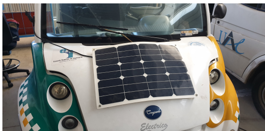
(a) Panel delantero instalado
