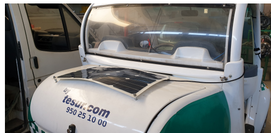
(b) Panel trasero instalado
