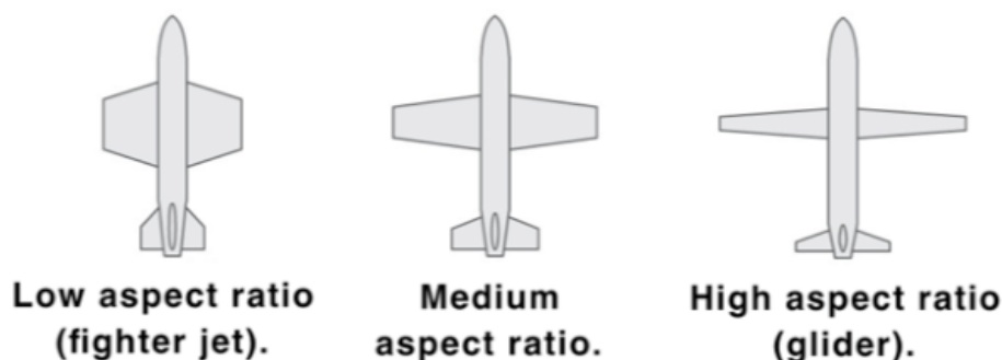
Figura 2.6. Alargamiento alar. Fuente: How wing design affects lift, Nicholas Landell-Mills.
